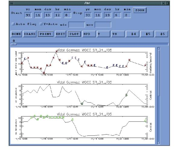
Figure 11. Screen shot of the VIDAT editor window with assigned QC flags displayed. Data for wind speed, air temperature, and sea temperature are shown for the 1993 SR-01 cruise of the R/V *Vidal Gormaz*
