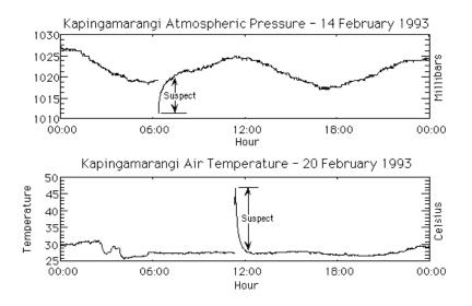
**Figure 16**. Examples of suspect pressure (a) and temperature data (b) on the island of Kapingamarangi in 1993. Regions between the arrows contain unlikely values that lacked supporting evidence for an instrument malfunction; thus they are flagged as suspect.
