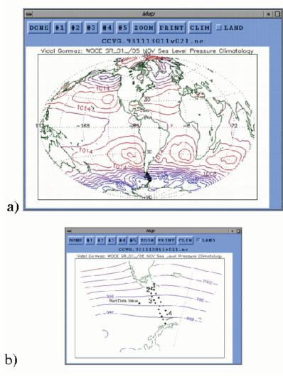
Figure 9. VIDAT screen shot of (a) the full globe cruise track map displaying the 1993 SR-01 cruise of the R/V *Vidal Gormaz* and (b) a zoom of the same cruise track showing an erroneous ship position value. Both panels display the atmospheric pressure climatology for November (da Silva et al. 1994).
