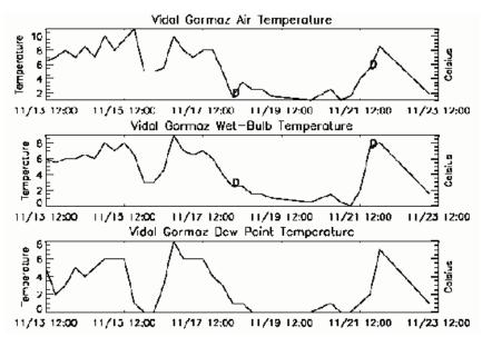
Figure 7. Dry air, wet-bulb, and dew point temperature data from the R/V *Vidal Gormaz*. The values flagged with a *D* failed the  $T^{\geq}Tw^{\geq}Td$  t test (see text).
