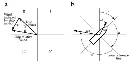
Figure 6. Schematic diagrams showing a) vector subtraction method of calculating the true wind and b) the six vectors and angles required to compute the true wind (T). In a) the roman numerals mark the quadrants in the cartesian coordinate system. (see text for more details)
