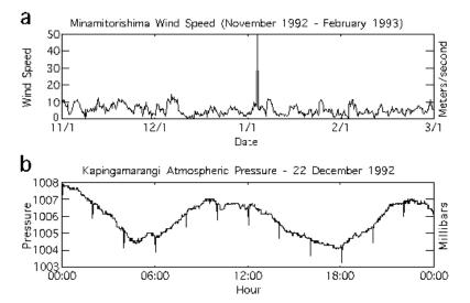
Figure 17. Examples of (a) a single large wind speed spike at Minamitorishima and (b) rhythmic one millibar atmospheric pressure spikes at Kapingamarangi. Both are flagged with an *S*.
