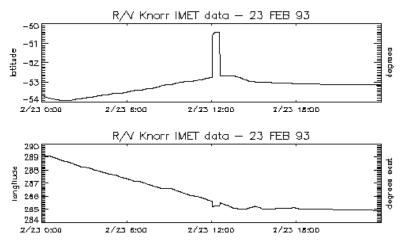
Figure 4. Rapid changes in latitude and longitude values, like these for the R/V *Knorr*, are flagged for failing the platform speed test. All values within a region of rapid change are flagged.
