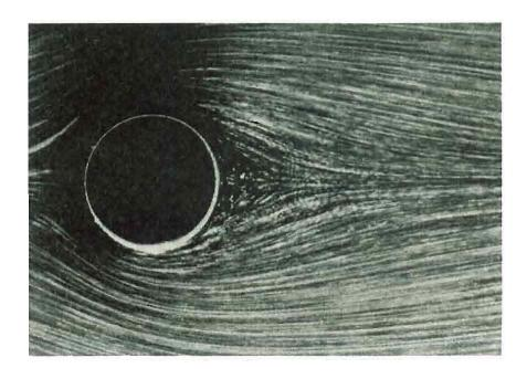
Fig. 4: Circular cylinder at R=9.6 (from Van Dyke 1982). It was developed by moving a cylinder through a tank of water containing aluminum powder and illuminated from underneath. *Photograph taken by Sadatoshi Taneda*.
