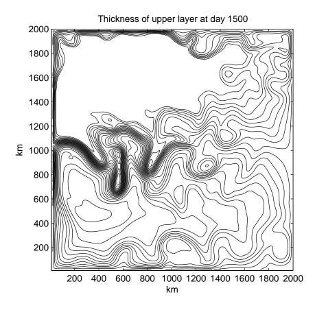
Figure 16: Contour plot of the thickness of the upper layer at day 1500. The contour interval is 10 meters. Over much of the northern region the lower layer wells up to the surface, so the thickness of the upper layer is near zero in such locations. The maximum and minimum computed thicknesses for the upper layer are approximately 244 and  $10^{-9}$  meters, respectively.
