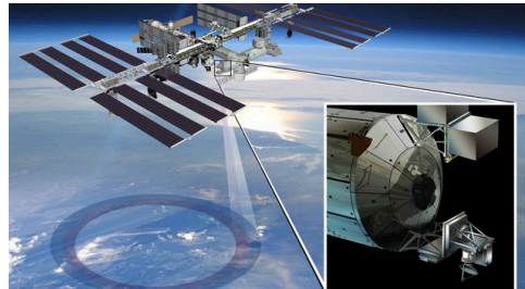
NASA's ISS-RapidScat satellite bounces microwaves off the ocean surface and measures the return pulses. Stronger signals mean rougher seas, caused by stronger winds. Ocean-wind data are critical for short- and long-term weather forecasts, tracking storms, analyzing climate trends and understanding the interplay of wind, ocean and sea life.
