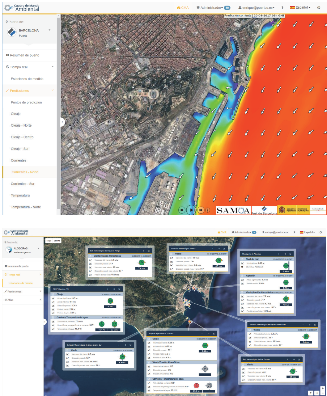
Figure 27.4. The SAMOA visualization tool, showing the circulation at Barcelona Port (upper panel) and the real-time measurements at Algeciras Harbour (lower panel).
