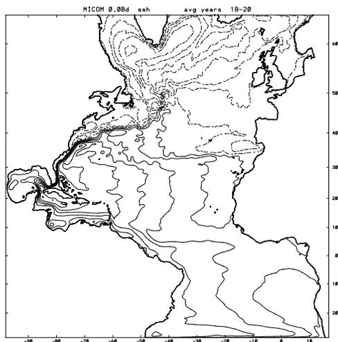
**Figure 1.** 3-year-mean model SSH field for the  $1/12^\circ$  COADS-forced MICOM. The viscosity operator is a combination of biharmonic ( $A_4 = V_D \Delta x^3$ , with  $V_D = 1$  cm/s) and Laplacian ( $A_2 = \max[.1 \Delta x^2 \times \text{deformation tensor}, V_D \Delta x]$ , with  $V_D = .5$  cm/s).
