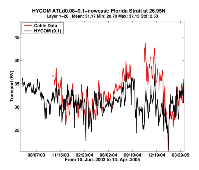
FIGURE 15. The transport in the Florida Current at 27°N from the 1/12° Atlantic near real-time system in black. Observed transport variations in the Florida Current are being monitored by measuring the cross-stream voltages using an undersea cable between Florida and the Bahamas. Daily transport data are available from March 1982 to October 1998, and from March 2000 onward (Baringer and Larsen, 2001). Observations from the cable data are shown in red.
