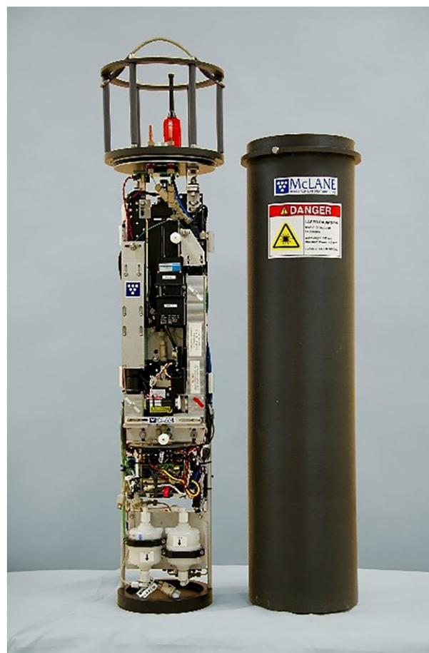
FIG. 19.15 The Imaging Flow Cytobot, an imaging microscope that can provide real-time sensing of harmful algal blooms. IFCB, McLane Research Laboratories, 2022a. Photograph used with permission.
