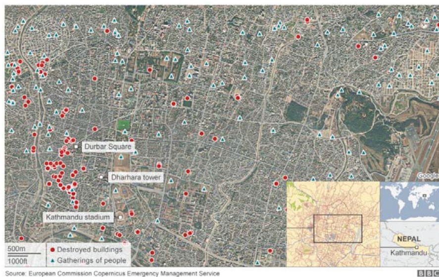
FIGURE 10.14 Repeated acquisitions of high resolution optical imagery provided details on destroyed buildings and other infrastructure following the 2015 M7.8 Nepal earthquake. The earthquake destroyed century-old buildings, killed nearly 9,000 people, and left hundreds of thousands homeless. The shaking also triggered numerous landslides, which contributed to widespread destruction of many small villages. The International Charter “Space and Natural Disasters” was invoked to enable space agencies to target space acquisitions in the damaged areas. SOURCE: Pleiades image, CNES.
