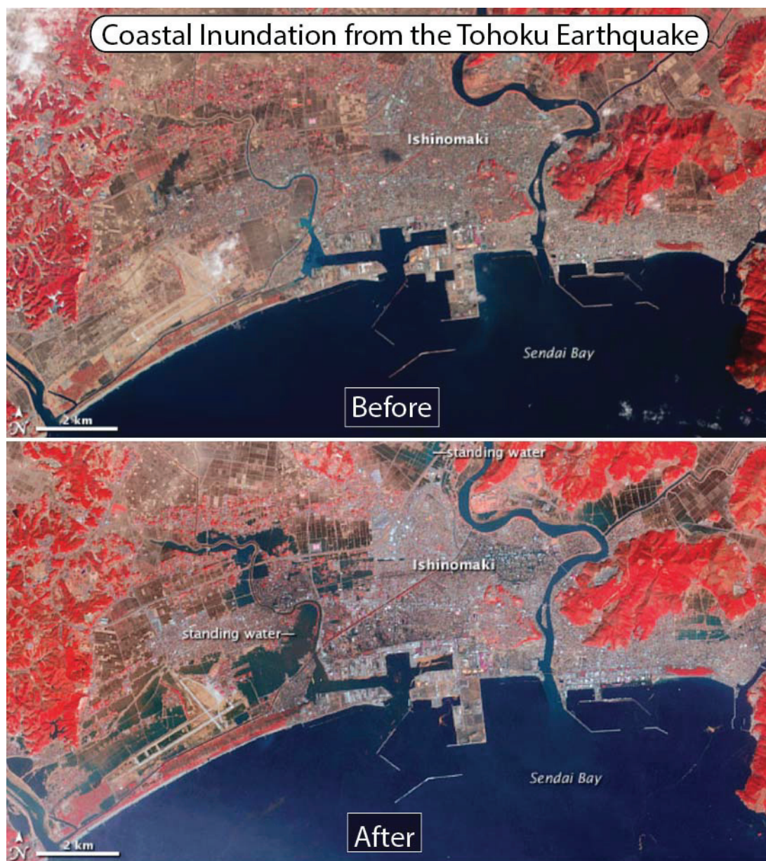
FIGURE 10.1 Coastal inundation in the Sendai Bay, Japan, region captured by the ASTER (Advanced Spaceborne Thermal Emission and Reflection Radiometer) satellite before and after the 2011 Tohoku earthquake and tsunami: the costliest natural disaster in history. SOURCE: Modified from NASA, https://earthobservatory.nasa.gov/Features/Gallery/tsunami.php .
